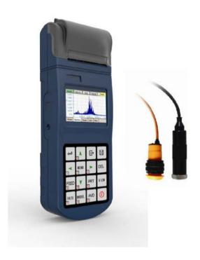
TMV500 uses piezoelectric acceleration transducer to convert vibration signal into electric signal. Then by analyzing input signal, results including RMS of velocity values, peak-peak value of displacement, peak values of acceleration or real-time spectral charts are displayed or printed out. It can not only measure the three parameters, but also for rotational speed measuring.
